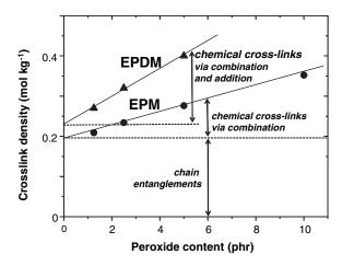
Figure 3. The total effective network density for EPM (without ENB) and EPDM with 2% ENB versus peroxide content. Since no chemical cross-links are formed without peroxide, the intercept of the plot reflects the apparent entanglement density. The entanglement densities of EPM and EPDM are not the same, probably because they have different conformational states as a result of their different chemical composition.
