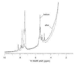
Figure 2. 12.5 kHz MAS  $^{1}$ H NMR spectra of EPDM (2% ENB, 5 phr peroxide) before and after peroxide cross-linking, reflecting a ENB conversion of  $\sim$ 50%.
